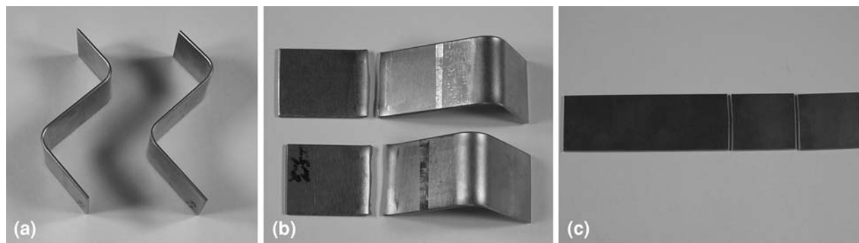
Fig. 10 Results of the double bend test samples from different sheet materials
